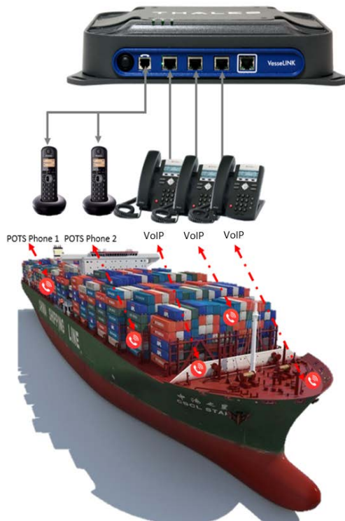
Figure 2-2 Local Communications via PBX Functionality
